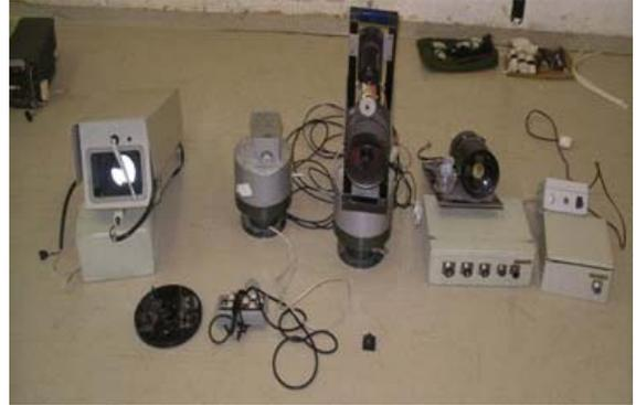
**A long-range observation system. Center: a long-range camera, to the left of which is a rotating and elevation system.**
