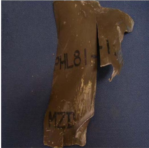
Part of the casing of a 122 mm cluster rocket warhead. The inscription PHL-81 identifies it as a Type 81 rocket of Chinese manufacture. Such rockets hit the Druze village of Maghar (See Footnote 3).
