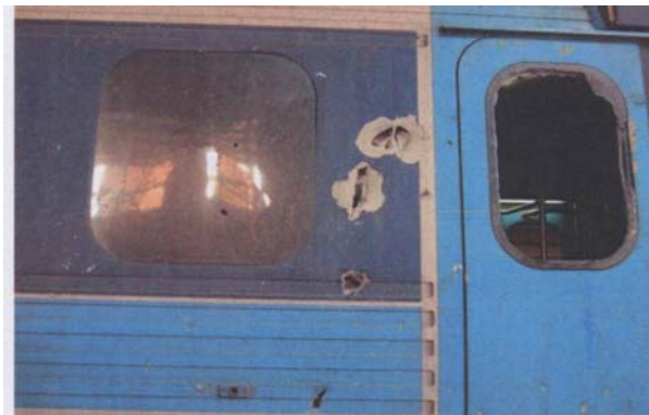
Ball-bearing hits in the side of a railroad car standing near the point of impact
