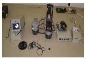
A long-range observation system. Center: a long-range camera, to the left of which is a rotating and elevation system.
